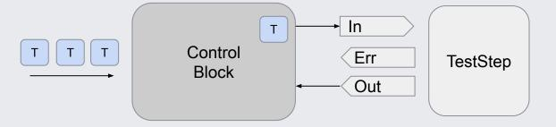
The TestRunner controls the flow of Targets through the TestSteps.
