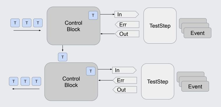
The TestRunner controls the flow of Targets through the TestSteps.
