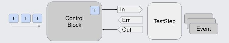
The TestRunner controls the flow of Targets through the TestSteps.
